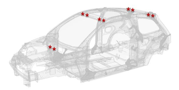
The smaller local RDM<sup>®</sup> "nuggets" are represented as spot-welds. A total of 10 were created which increased the body stiffness by 1% for no mass change.
