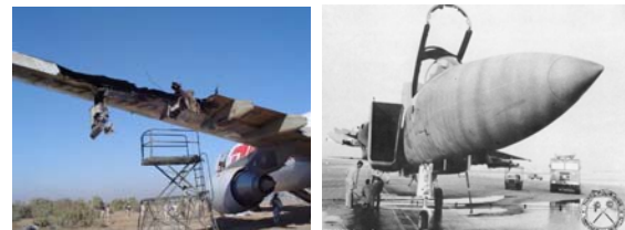
Fig. 2 In-flight damaged A-300-600 aircraft (left) and F-15 aircraft starboard wing damage due to mid-air.
