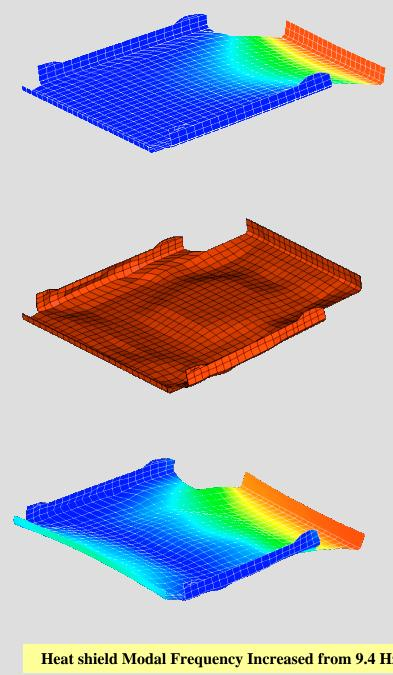
1<sup>st</sup> Bending Freq = 9.4 Hz. For Flat Heat shield
