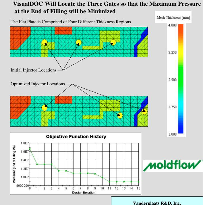
Identify Injector locations to minimize the pressure
