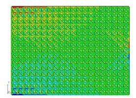
Cycle O Loadcase 1 Bar Force Axial End A
