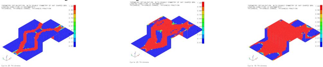
Figure 12. Topometry Optimization results. Red: Thickness=1.0, Blue: Thickness=0.01 a) Volume \leq 600 mm 3 (Mass fraction \leq 0.25 ) b) Volume \leq 1200 mm 3 (Mass fraction \leq 0.50 ) c) Volume \leq 1800 mm 3 (Mass fraction \leq 0.75 )
