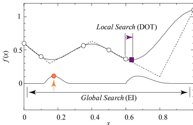
Figure 4. Schematic of Kriging-DOT optimizer
