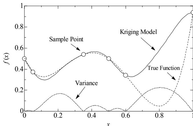
Figure 1. Schematic of Kriging Model.
