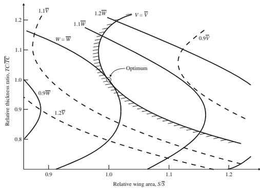
**Figure 4. Design Space Using Wing Area as a Design Variable**
