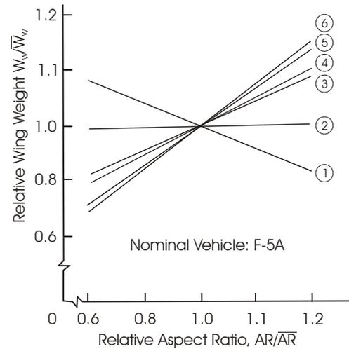
Figure 1. Wing weight Versus Aspect
