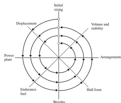
**Figure 5. The Ship Design Spiral**
