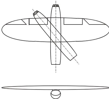
Figure 2. All Wing Remotely Piloted Vehicle
