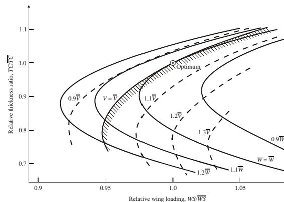
Figure 3. Design Space Using Wing Loading as a Design Variable
