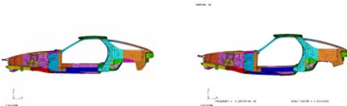
**Figure 1. First Natural Bending mode**
