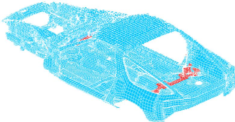
Figure 5. Average of First Torsion and First Bending Frequencies Maximization Results
