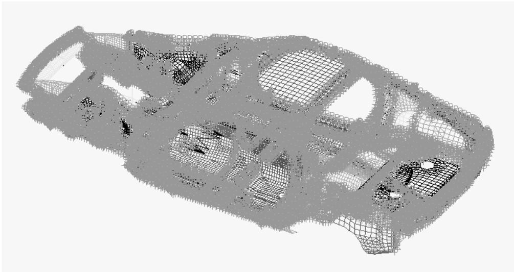
**Figure 14. Weld Optimization Model of Car Body**
