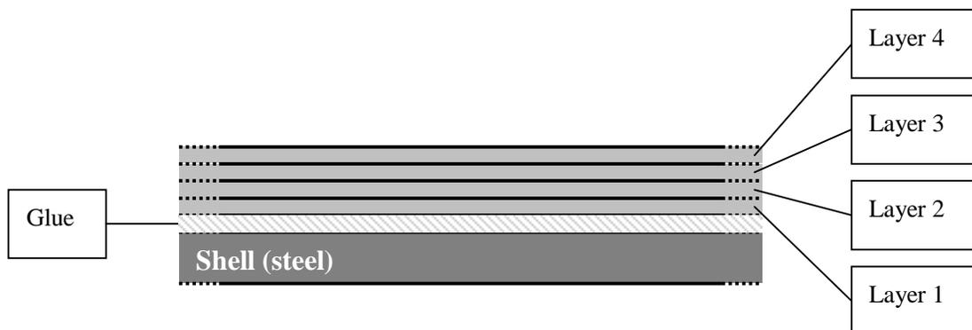
**Figure 7. Section of a Patch**
