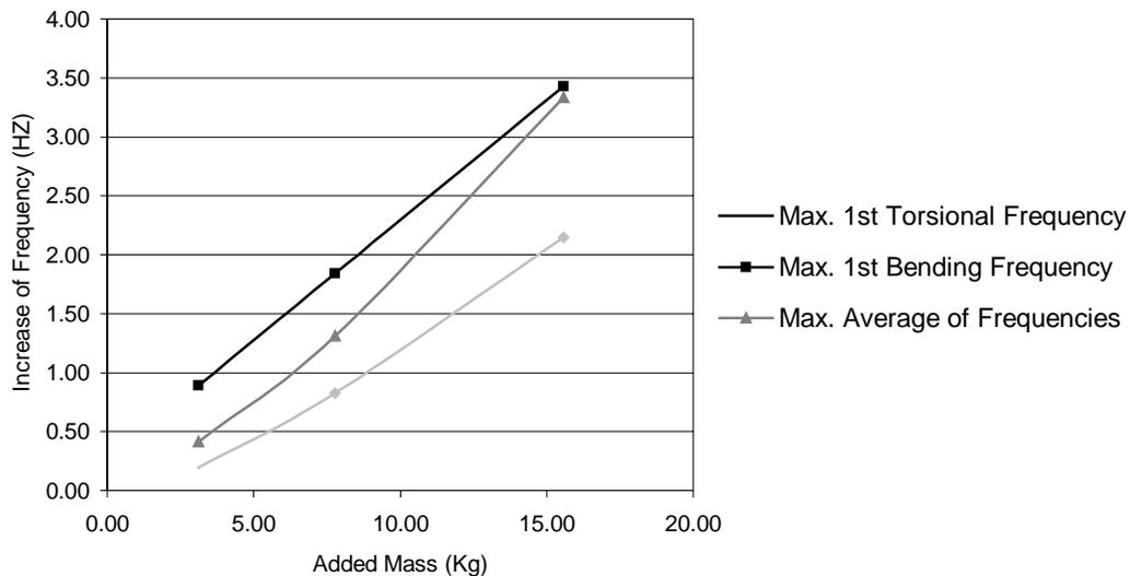
**Figure 6. Relation Between Increased Frequency And Added Mass**
