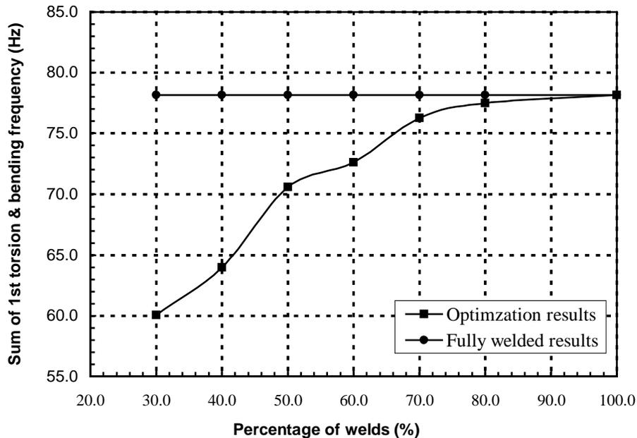
**Figure 18. Relation Between Rigidity and Number of Welds**
