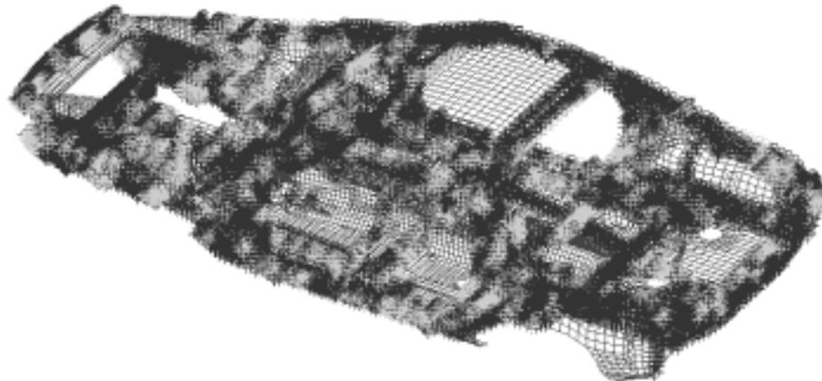
**Figure 15. Optimal Result with 70% Retained Welds and 30% Removed Welds**
