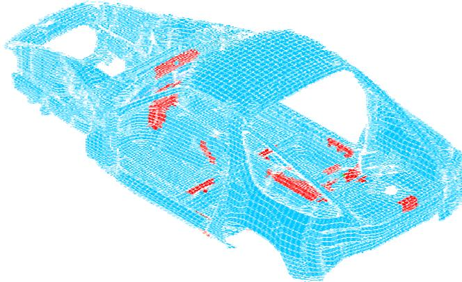
Figure 4. First Torsion Maximization Results
