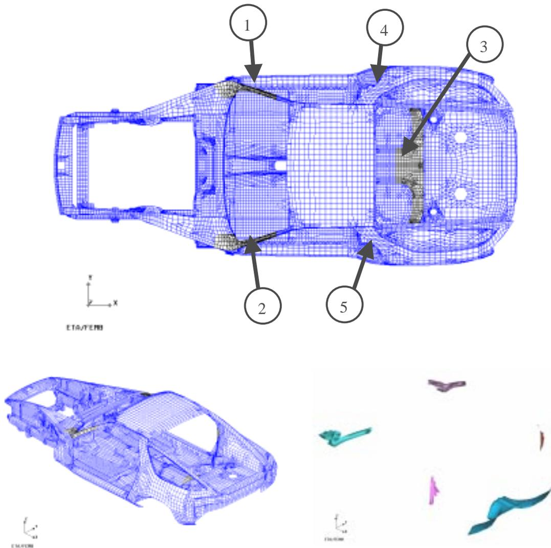
**Figure 12. Patches for First Torsion Frequency Optimization**
