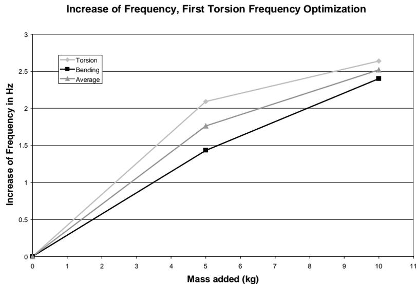
Figure 11. Frequency Increases for Different Mass Constraints
