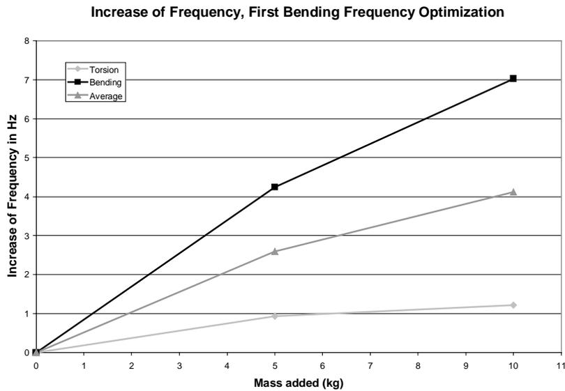
Figure 9. Frequency Increases for Different Mass Constraints
