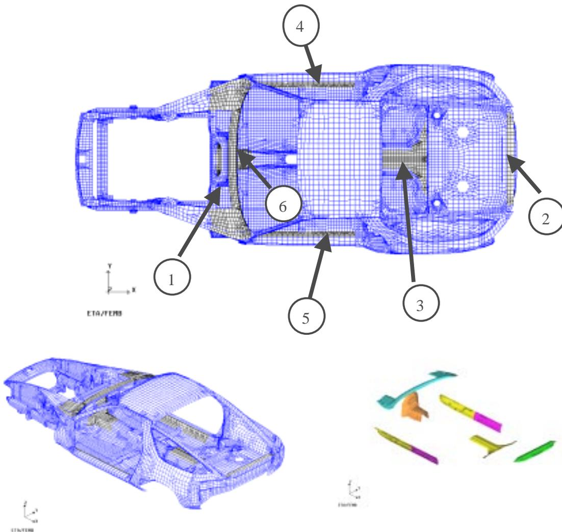
**Figure 10. Patches for First Torsion Frequency Optimization**
