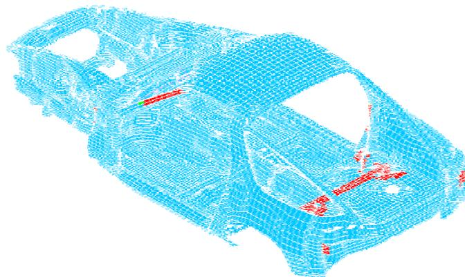
**Figure 3. First Natural Bending Maximization Results**
