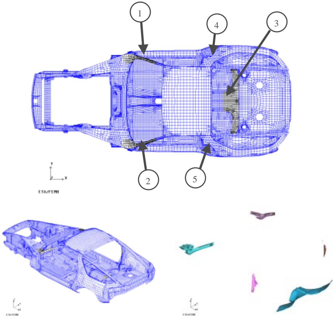
**Figure 8. Patches for First Bending Frequency Optimization**
