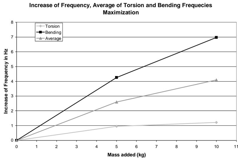
Figure 13: Increase of Average of First Bending and Torsion Frequencies Maximization
