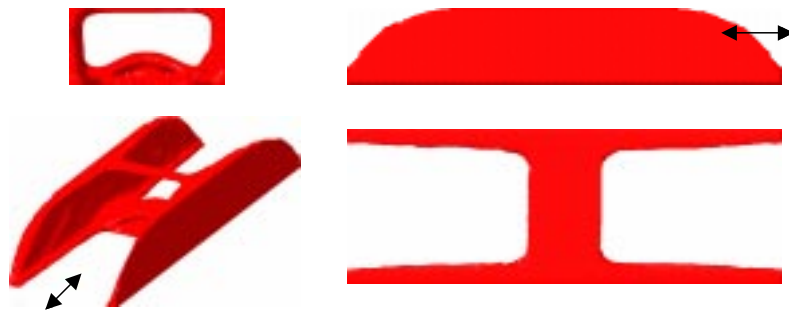
Figure 11. Topology Results for Casting in the Y Direction
