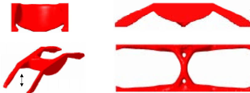
Figure 9. Topology Results for Casting in the Z Direction
