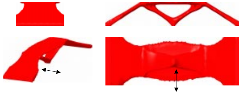
Figure 10. Topology Results for Casting in the X Direction
