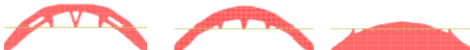
Figure 14. Topology Results with Quadrilateral Elements: Standard, Casting with variable parting Surface and Casting With Fix Parting Surface on Bottom
