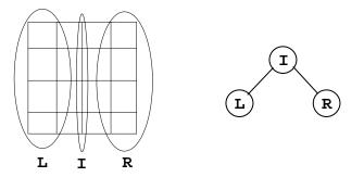
Each circle in the graph is a supernode that represents several nodes of the FE model. The **L** and **R** partitions can be further divided, and a new elimination tree generated as shown in the following figure:
