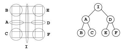
The SMS method contains powerful heuristics to automatically partition a structure into thousands of supernodes in an elimination tree that has dozens of levels.
